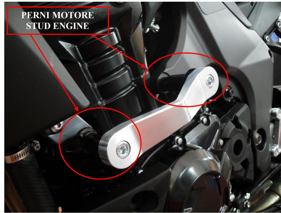
To mount the bracket 4Racing buffer over, unscrew the bolts and screw motor 1 at a time on the pad bracket.
